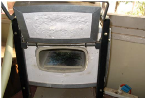
Photograph 02: SMF lagged kiln
